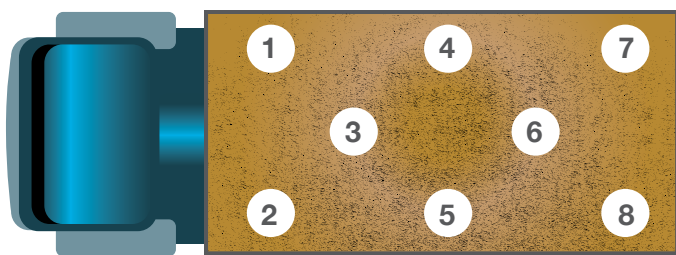
Figure 7. A 30-tonne grain lorry should have 8 evenly spaced samples taken
